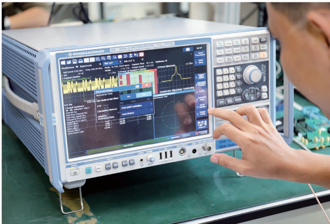
NB-IoT RF transceiver test 窄帶物聯網射頻收發器測試
